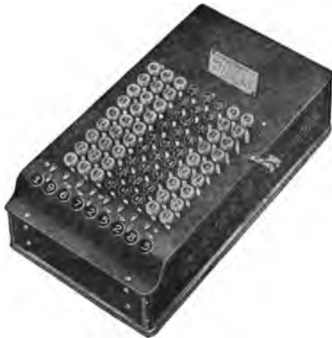
Fig. 25.—Adding and Multiplying Machine.
